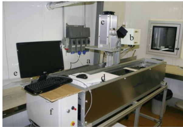
Fig. 1: Image of the hyperspectral system consisting of: a) high-precision linear stage with samples holder and motor driver; b) HeadWall camera; c) halogen lamp; d) calibrated Lambertian Spectralon ® panel useful to calculate reflectance; e) PC connected to the spectrometer through a dedicated interface; f) Single-Board RIO with Ethernet TCP/IP wireless connection – Credit: Garzonio et al.
